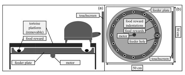
Fig. 1. Tortoise touchscreen apparatus: (a) side view of the Skinner box, (b) top view of the feeder plate (illustrations not drawn to scale).
